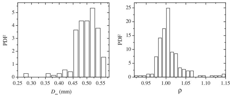
Fig. 2. Characterization of  $\text{Li}_4\text{SiO}_4$  pebble geometry. Left: pebble size distribution; right: pebble shape distribution.
