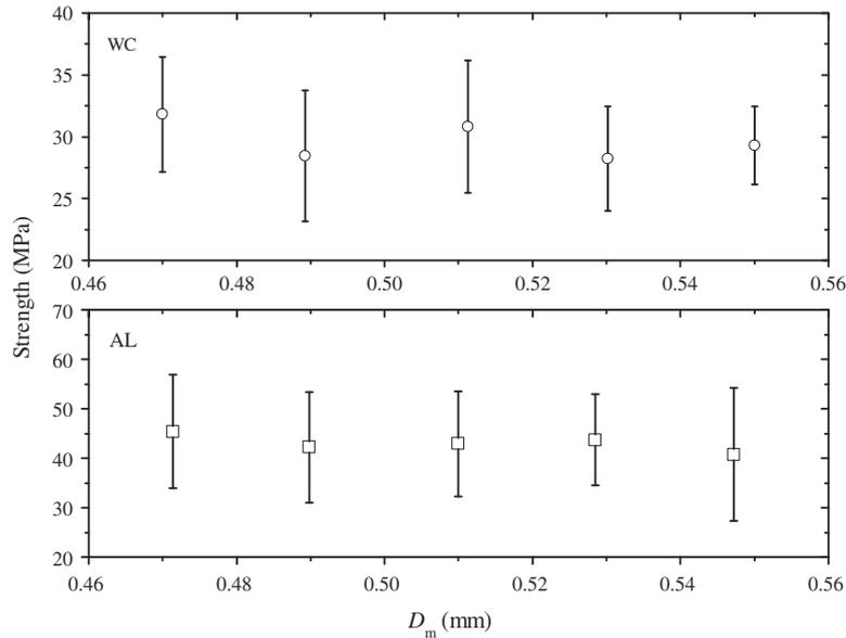
Fig. 3. Size effect of the contact strength  $F_c/D_m^2$ . Top: compression by WC plates; bottom: compression by AL plates.
