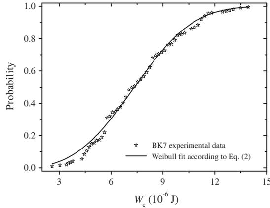
**Fig. 8.** The energy strength distribution of conditioned pebbles from the batch OSi 07/1 in dry inert gas environment. Fitting parameters:  $W_{\text{Mat}} = 8.2 \times 10^{-6}$  J and  $m = 3.2$ . The deviation of these values from the ones obtained at air indicates the significance of the influence of the environmental conditions.
