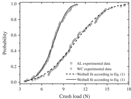
Fig. 4. Crush load distributions for single  $\text{Li}_4\text{SiO}_4$  pebbles in air.
