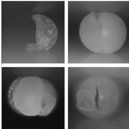
Fig. 6. Some failure forms of  $\text{Li}_4\text{SiO}_4$  pebbles.
