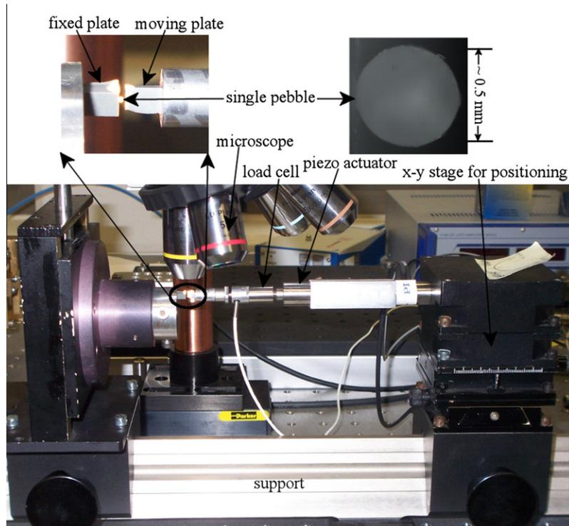
**Fig. 1.** Experimental apparatus for single pebbles in air.
