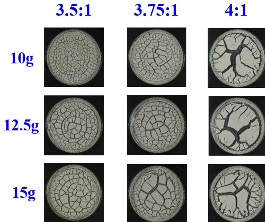
**Figure 1. Crack patterns of the drying film with different weight of solid and different mass of water**
