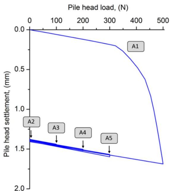
Fig. 3: Pile head load-displacement curve
