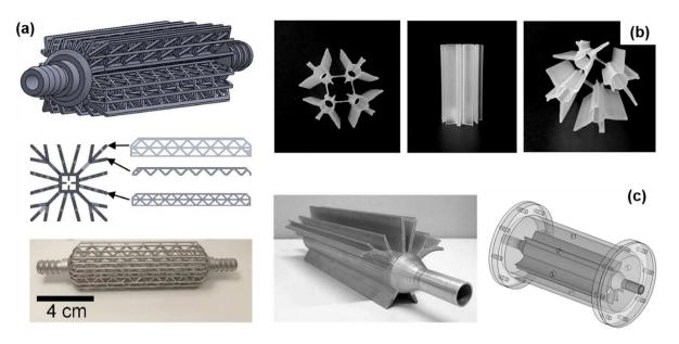
**Figure 11.** Additive manufactured fins and extended surfaces: (a) Additive manufactured device with external and internal fins to enhance heat transfer [71] (b) Additive manufactured multi-tube device with an optimised fin configuration [16] (c) Additive manufactured optimised fin configuration for melting performance enhancement [160].
