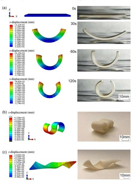
**Figure 9.** Four-dimensional-printed ABS objects with the FEM simulations: (**a**) the concave design; (**b**) the wave design; (**c**) the spiral design. The colour scale bars are different for each figure as their function is to indicate the level of deformation at each stage.
