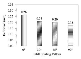
Figure 7. Deflection of the rectangular bars printed with different infill patterns.
