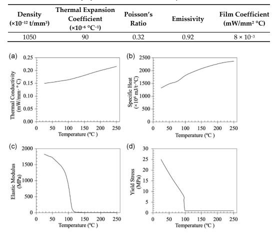
Table 1. Common material properties of ABS used in FEM analysis.
