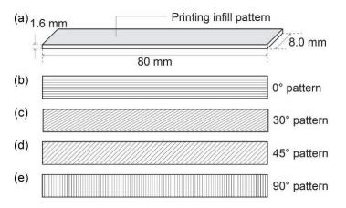
**Figure 3.** Simulated geometry and printing patterns of the rectangular bars for the FEM analysis: (a) the dimensions of the rectangular bar; (**b**–**e**) the infill printing patterns.
