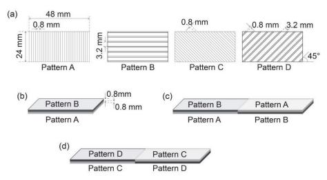
**Figure 4.** Design of the printing patterns of 4D-printed objects: (**a**) the four basic printing patterns with different raster angles; (**b**) the combination of the printing patterns to achieve the concave design after heat treatment; (**c**) the combination of the printing patterns to achieve the wave design after heat treatment; (**d**) the combination of the printing patterns to achieve the spiral design after heat treatment.
